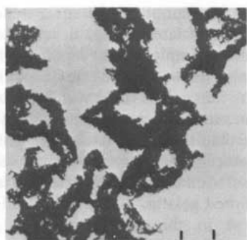
Figure 3: Different halides have somewhat different filament growth patterns. Left to right: AgCl, AgBr, AgI
