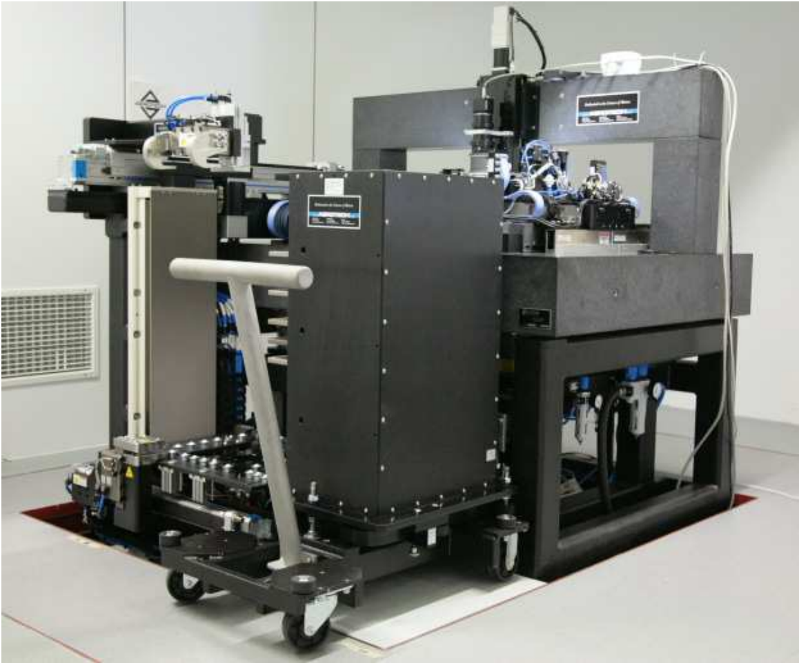
DAMIAN digitiser with automatic plateloader and mobile platewagon
